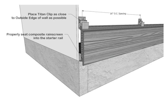
Important Note\* If your board does not seat properly, don't install it. NEVER "force" a board into place. You may cut out any bow or bend (defect cutting) and install only the usable portion of the siding board.
