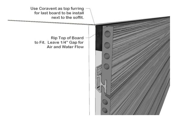
Note\* If you trim the width ¼" narrower than required, it will be easier to install the siding and allows for better ventilation at the top of the rain screen wall cavity.
