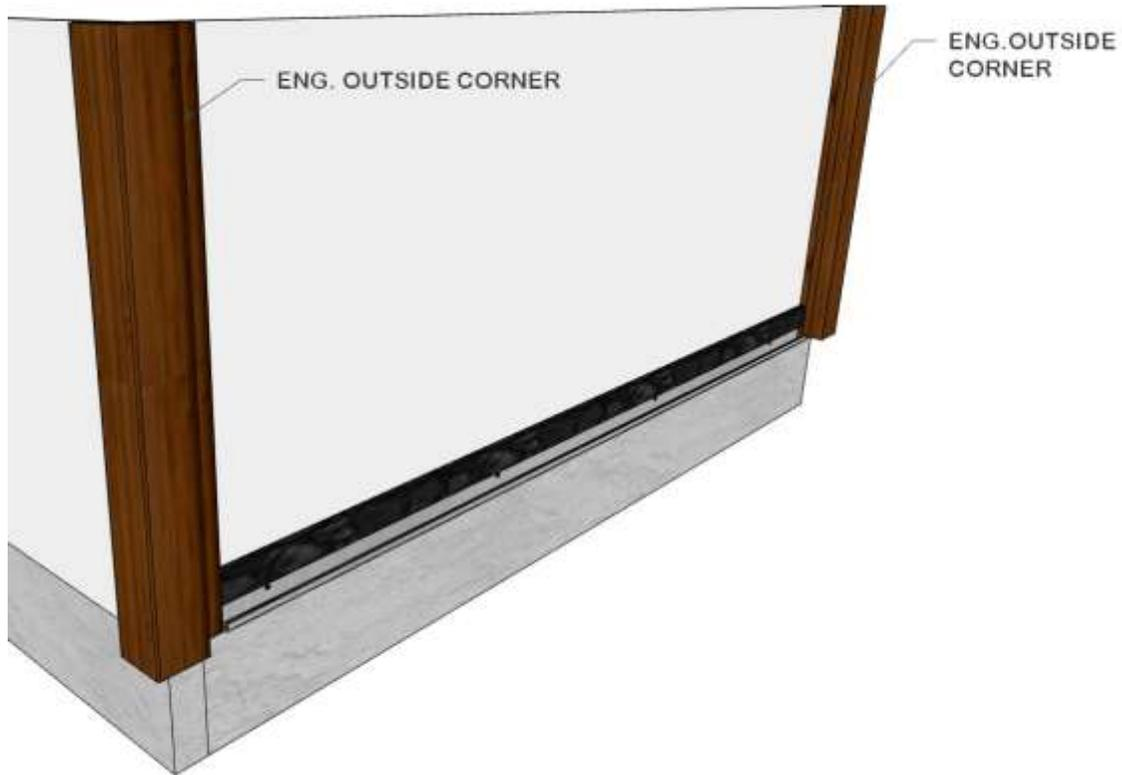
**\*\*NOTE:** Outside corners are typically mitered onsite. An 18-gauge brad nail can be used to help secure outside corners to keep them stable and in place. It is also recommended that Lamboo Titan Clips are positioned as close to the outside corner to help with maintaining closure and uniformity of the mitered corners.
