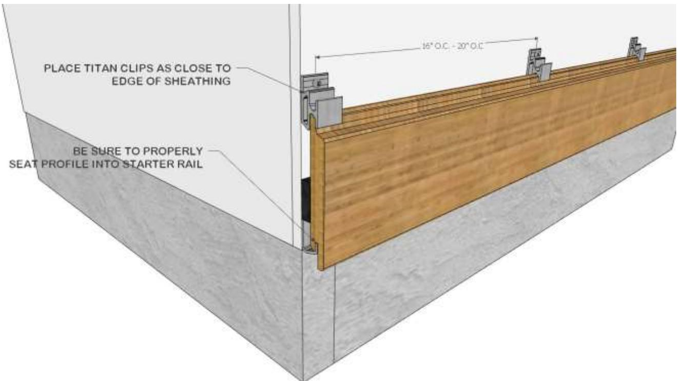
*Important Note\* If your board does not seat properly, don't install it. NEVER 'force' a board into place. You may cut out any bow or bend (defect cutting) and install only the usable portion of the siding board.*
