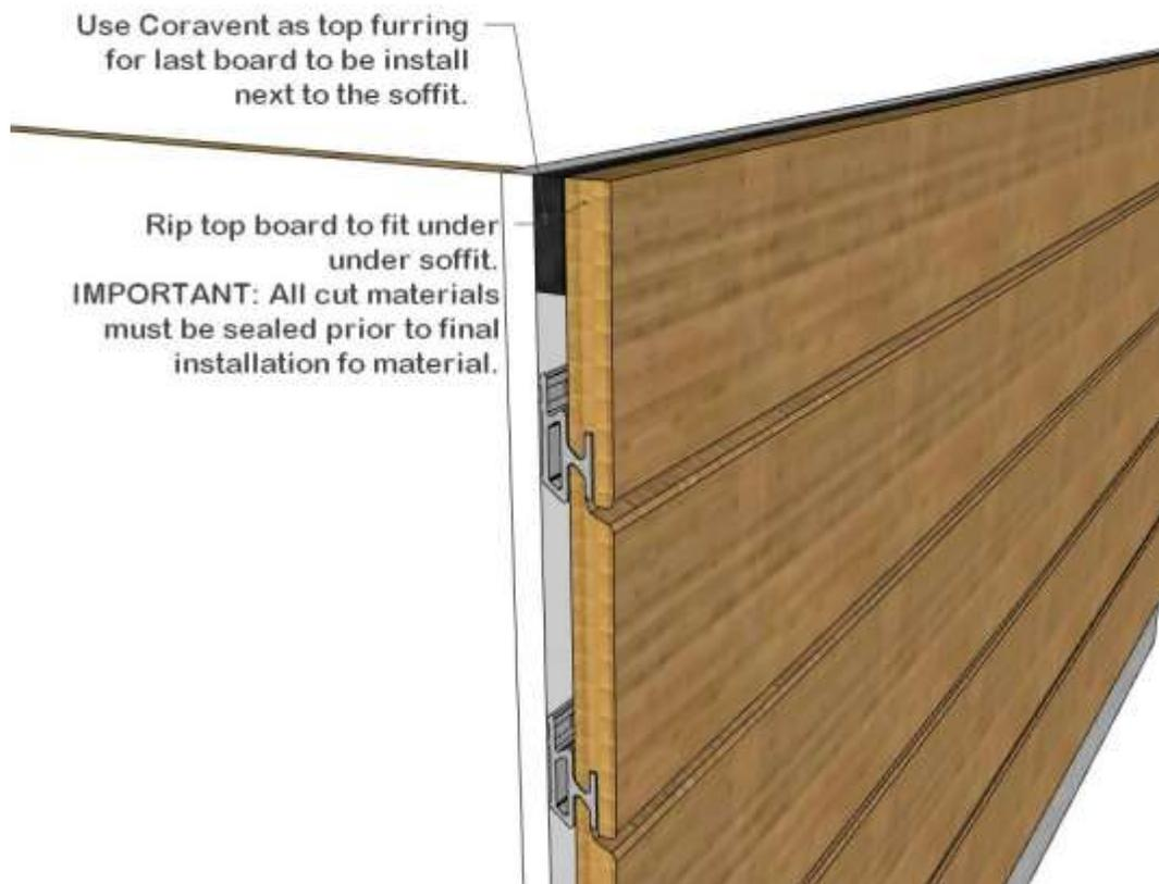
*Note\* If you trim the width ¼" narrower than required, it will be easier to install the siding and allows for better ventilation at the top of the rain screen wall cavity.*
